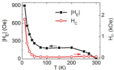
FIG. 2. Temperature dependence of the (a) coercive field,  $H_C$ , and (b) absolute value of the exchange bias field,  $H_E$ , for the 7.5-nm FeMn layers sample whose hysteresis curve is shown in Fig. 1. The line is a guide to the eye.
