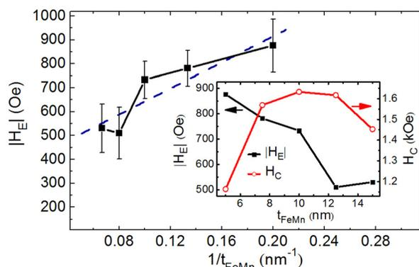
FIG. 4.  $H_E$  vs. inverse thickness,  $1/t$ , of FeMn for the same samples as in the inset. The dashed blue line is a linear fit. Inset: Dependence of the coercive field,  $H_C$ , and absolute value of the exchange bias field,  $H_E$ , on the thickness of FeMn for FeMn/Cu multilayers. The line is a guide to the eye.
