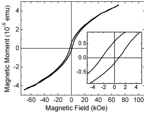
FIG. 1. Hysteresis loop measured at 10 K for the FeMn/Cu sample with 7.5-nm FeMn layers.  $m_R = 0.38 \cdot 10^{-5}$  emu,  $M_{7T} = 4.6 \cdot 10^{-5}$  emu,  $H_E = -782$  Oe,  $H_C = 1569$  Oe. Inset: the central portion of the hysteresis loop.
