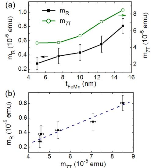
FIG. 3. (a) Magnetic moment of the samples at  $H = 7$  T,  $m_{7T}$ , and the remanent magnetic moment,  $m_R$ , as a function of FeMn thickness; the line is a guide to the eye. The error bars for  $m_{7T}$  are smaller than the circles used for the data points. (b) Correlation between the two magnetic moments in (a); the dashed blue line is a linear fit.
