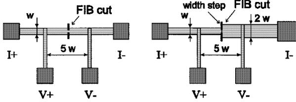
Fig. 2. Sketch of two types of single wires with a FIB-fabricated constriction.
