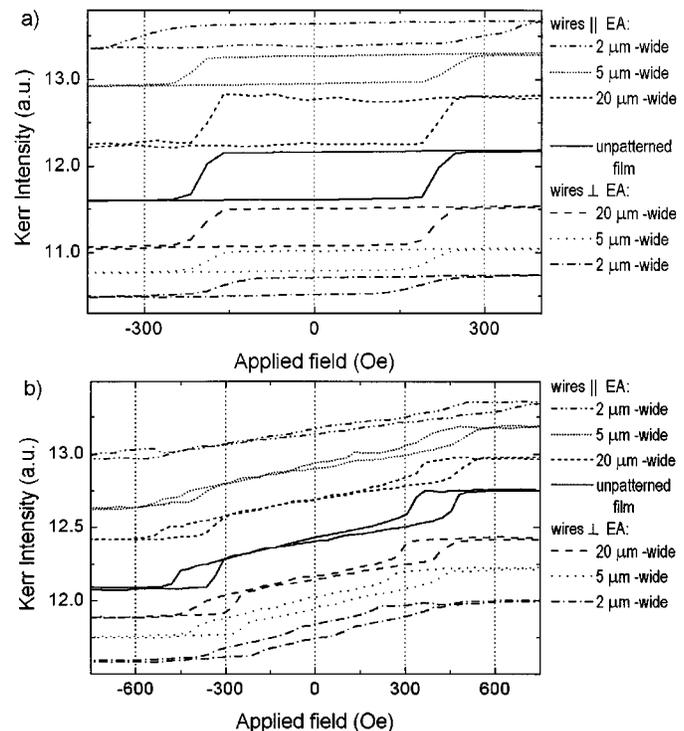
Fig. 1. MOKE measurements: Magnetization of 25 nm-thick unpatterned epitaxial Fe film and wires oriented parallel and perpendicular to the easy magnetic axis when (a) the magnetic field is applied along the easy axis; (b) the magnetic field is applied perpendicularly to the easy axis.
