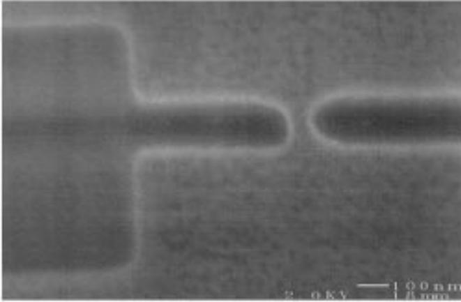
Fig. 3. SEM image of a typical sub-100 nm cut [same as in Fig. 4(b), rotated by 90°] fabricated with FIB in a 25 nm-thick Fe wire. The scale bar is 100 nm.
