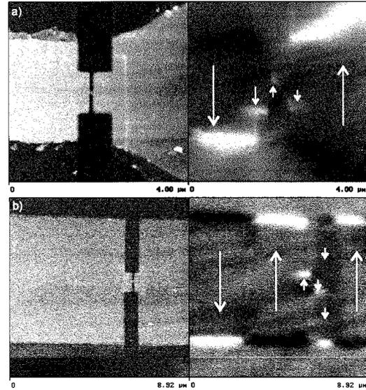
Fig. 4. AFM (left) and zero-field MFM (right) images of typical sub-100 nm cuts fabricated with FIB in a 25 nm-thick, nominally 5  $\mu\text{m}$  (a) and 2–4  $\mu\text{m}$ -wide (b) Fe wires with a domain wall trapped (a) in the middle of the cut, (b) at the left side of the cut.
